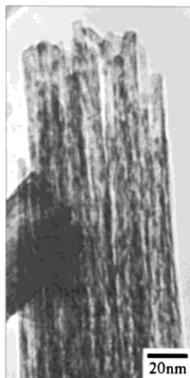
Figure 1. TEM micrograph of hematite nanorods, self-assembled as a bundle.
